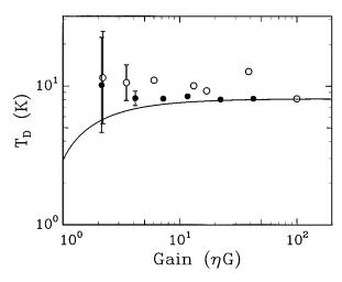
FIG. 1. The difference between the pump-on noise and the reference noise referred to input using the single sideband power gain  $\eta G$ . The error bars indicate uncertainty in the data due to detector saturation effects. Open circles represent data taken below threshold; filled circles represent data taken above threshold. The solid curve represents the theoretical prediction.
