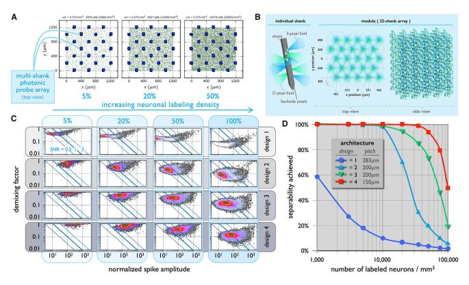
Figure 8. Computational Approach to De-mix Detector Photon Counts to Obtain Multiplexed Time Records of Individual Neuron Activity (A) Schematic depicting a top view of one 24-shank photonic probe array module (design 1), implanted in a 0.558 mm<sup>3</sup> volume of mouse cortex that is labeled with increasing density.
