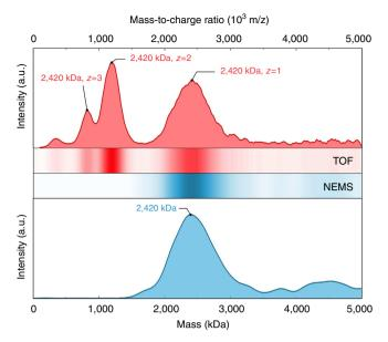
**Figure 2 | NEMS-MS greatly clarifies the spectrum.** Spectra for a nanocluster population with a mean mass of around 2,420 kDa acquired by both TOF and NEMS-MS. The TOF data was smoothed by applying a Savitsky-Golay filter. While multiply charged particles generate several peaks in the TOF-MS spectrum, the NEMS directly weighs the particle masses, yielding a single peak.
