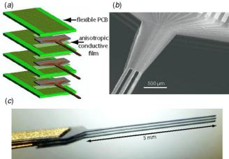
**Figure 6.** (*a*) Flip-chip assembly scheme for connecting the silicon devices with PCBs. (*b*) SEM micrograph of the rear section of a 50  $\mu$ m thick shaft array showing the multilayer stacked structure. Adjacent layers have a spacing of 100  $\mu$ m, which is set by the thickness of the flexible cable. (*c*) Side view of the 50  $\mu$ m thick shaft array showing that the shafts are stress balanced and are able to retain approximately constant relative spacing.
