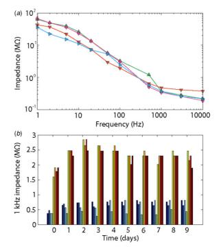
**Figure 8.** (*a*) Impedance versus frequency of four electrodeposited gold electrodes. (*b*) Electrode impedance measured over the course of 9 days for plated (left half of set) and unplated (right half) recording sites. Uncertainty in measured impedance is  $\sim 5\%$ .
