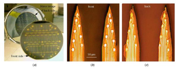
**Figure 4.** (*a*) The dual-side fabrication process is implemented on a 50 mm wafer. The transparent quartz carrier wafer is not visible. (*b*) Front and (*c*) back views of a representative finished device showing identical patterns. The overhanging structures on the left side of the shafts in (*c*) consist of SiO<sub>2</sub> that is displaced by up to 10  $\mu$ m from the Si shaft due to slight misalignment of features between the front and backsides.
