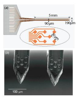
**Figure 2.** (*a*) Structure of a typical neural probe. This device contains two 5 mm long shafts. The inset shows the recording electrode arrangement. (*b*) SEM image of the tip of a fabricated probe. The gold electrodes have an area of  $100 \ \mu m^2$ , and the shafts have a thickness of 50  $\mu m$ .
