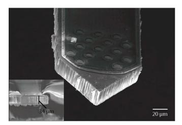
**Figure 5.** SEM micrograph of the tip of a dual-side neural probe. The total thickness of this structure, indicated by the cross-sectional view in the inset, is  $34 \pm 1 \mu$ m, which includes the ultra-thin substrate (~28  $\mu$ m before oxidation, manufacturer's specification =  $25 \pm 5 \mu$ m) and a stack of 2  $\mu$ m thick thermal oxide and  $3 \pm 1 \mu$ m thick parylene-C film on each side.
