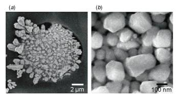
**Figure 7.** (*a*) Electron micrograph of a gold-electrodeposited microelectrode after a 9 day PBS immersion test. This site had an impedance of 0.65 M $\Omega$  on the final day. (*b*) Close-up of the surface of an electrodeposited electrode.
