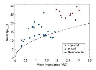
**Figure 10.** Root-mean-square noise at the electrode–fluid interface as a function of the mean impedance. The measurement bandwidth is 100–7000 Hz, and uncertainty in Z and  $\delta V$  is ~10% (error bars not shown). Blue circles and red diamonds represent electrodeposited and unplated gold electrodes, respectively. The thermal noise for a resistor with R = Z is also calculated (dashed line).
