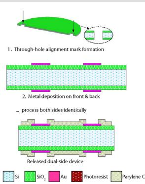
**Figure 3.** Modified process flow for fabricating dual-side devices on ultra-thin silicon substrates. The etching of through-holes is essential for achieving precise front-to-back feature alignment. Once metal has been evaporated on both sides, the parylene and oxide etch processes are carried out twice before the final DRIE step. The recording sites contain separately addressable leads on each side.
