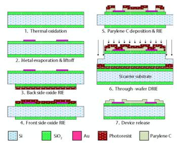
**Figure 1.** Fabrication process flow for single-side neural probe array built from ultra-thin silicon substrates. Each step relies on the use of a rigid supporting wafer to maintain structural integrity of the device substrate.
