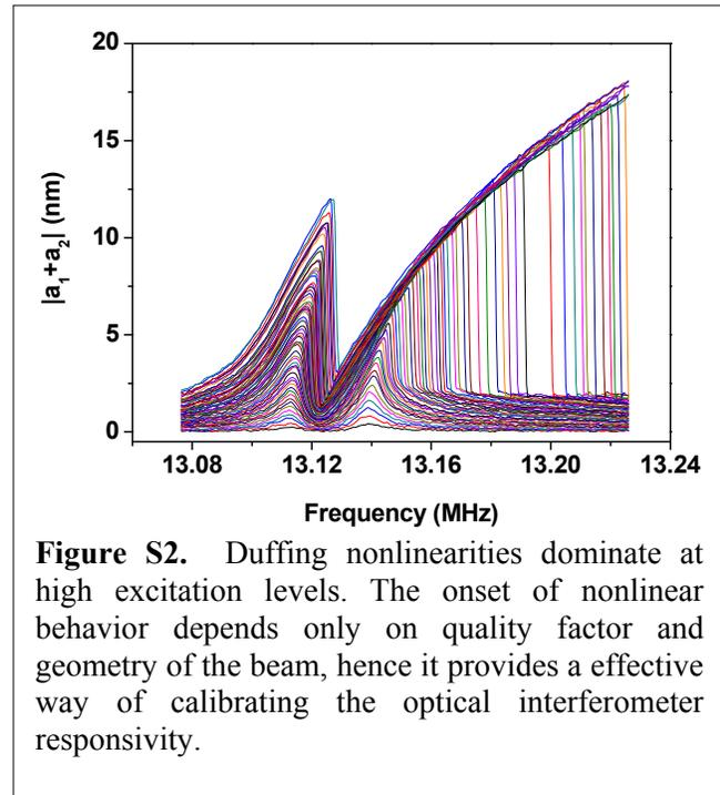
due to slight variations in their actuation efficiencies. The family of curves displayed represents drive amplitudes from  $50\text{mV}_{\text{rms}}$  to  $1.2\text{V}_{\text{rms}}$ . The onset of nonlinearity occurs for a  $\sim 600\text{mV}_{\text{rms}}$  drive level, which yields an optical signal of approximately  $70\mu\text{V}_{\text{rms}}$ . The estimated accuracy of this calibration is of order 10%.
