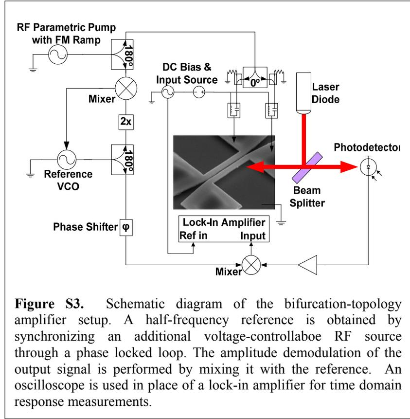
the pump and reference generators, an error signal is developed by homodyne converting the doubled reference output against the pump signal. The reference signal generated in this manner serves as the local oscillator for homodyne conversion of the photodetector’s radio frequency output signal. The reference phase  $\phi_{LO}$  is set by a phase shifter to maximize the mixer’s phase-sensitive baseband output.
