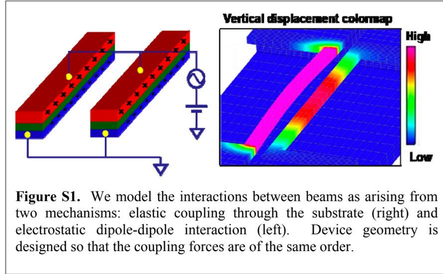
Electrostatic Coupling. When a DC bias voltage is applied to both beams, charges of opposite sign accumulate on their top and bottom surfaces forming dipole moments. Two such identical dipoles interact electrostatically with a force (3)
