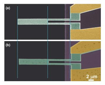
FIG. 6. (Color online) SEM micrographs showing two devices that were designed to have an identical aspect ratio of 7. Slight differences due to alignment mismatch can be observed. The nonlinear response of these devices (a) is presented in Figs. 5(a) and 5(c), while the nonlinear response for device (b) is given in Figs. 5(b) and 5(d).
