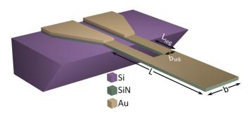
FIG. 1. (Color online) Schematic showing the type of device investigated in this study: a U-shaped cantilever beam of total length L and width b. The region close to the anchor presents two legs of length  $L_{\text{leg}}$  and width  $b_{\text{leg}}$ .
